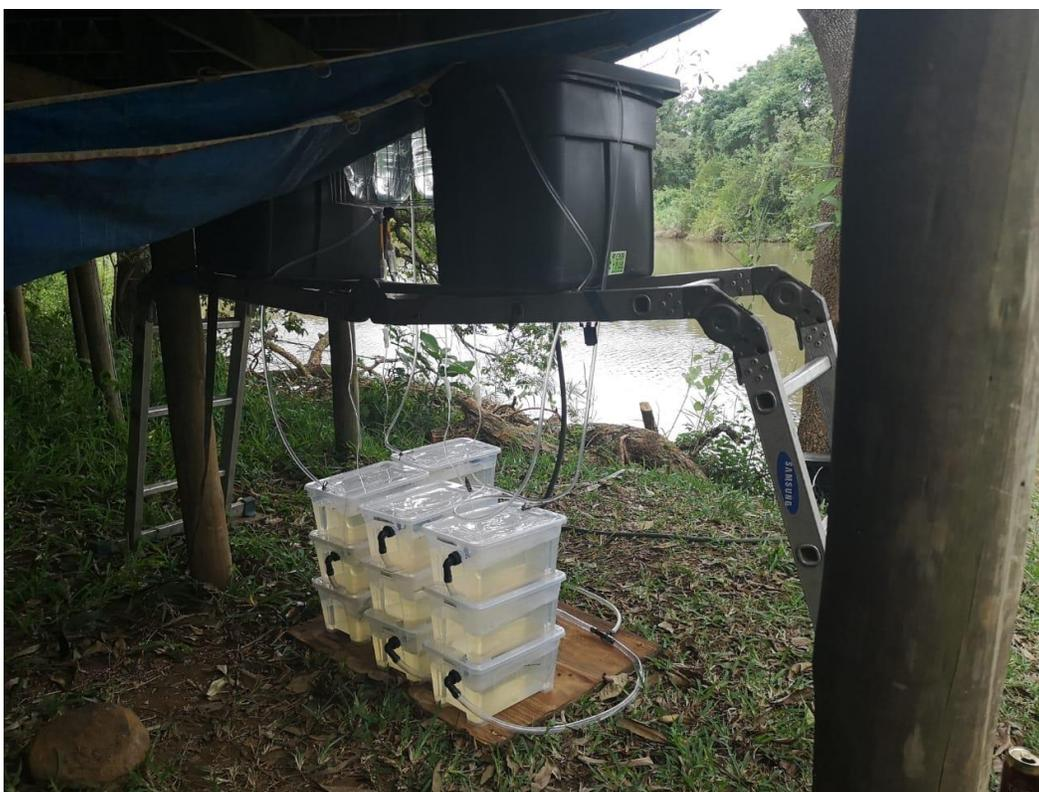
**Figure 1:** The water treatment system used to assess the efficacy of Prosol Agrigrow against *Phytophthora* and *Pythium*
